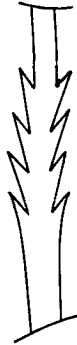
FIGURE 2. Form of breakdown near the nozzle at low flow rates: the shearing puffs, mode (a) of table 1.
